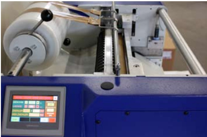
Compact construction: display, foil unrolling, forward feed unit and cutting system are grouped together in the smallest space.
