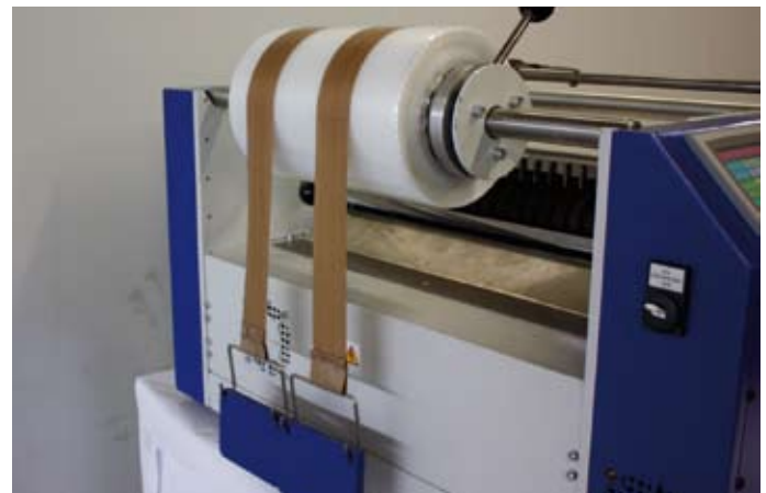
Simple and effective: braking bands with weights prevent unintentional unrolling of the film.
