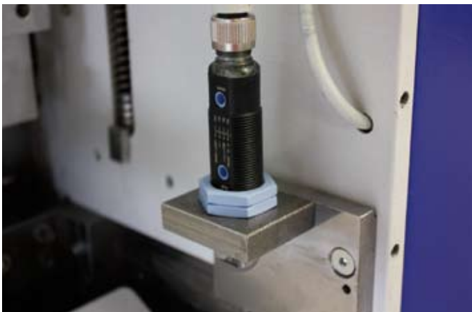
A photoelectric cell as protection against trapping. Safety first.
