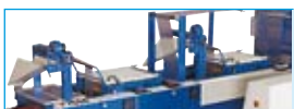
Automatic film sealing machine to manufacture PE gloves directly on a paper base
